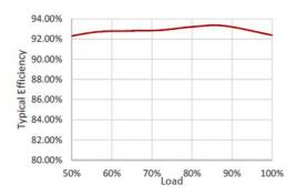
OT FIT 150 220-240 24 PC Typical Efficiency vs. Load
